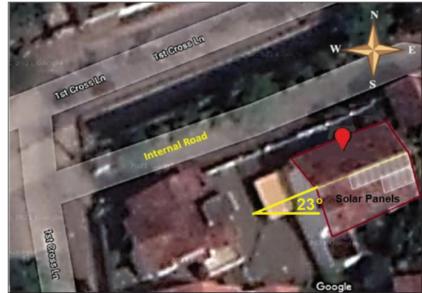
Figure 3: Orientation of solar panels on roof
