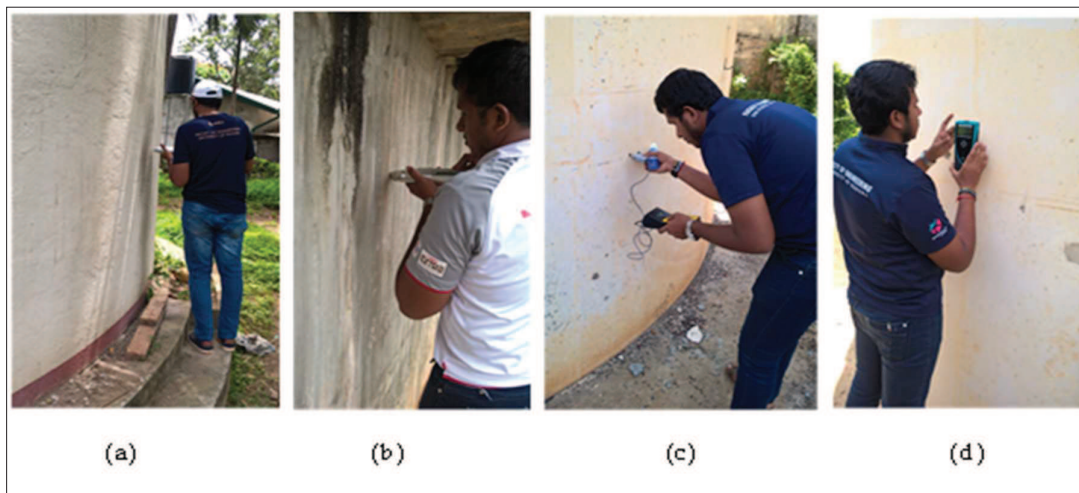
Figure 3: Data collection by NDT: (a) record data from visual inspection; (b) rebound hammer test; (c) concrete resistivity test; and (d) cover meter survey
