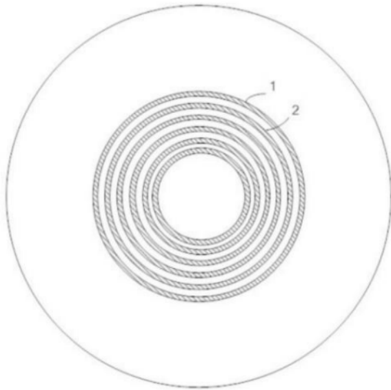
Figure 2. Within the specific aperture range of the lens, the annular micro-cylinder array is centred on the geometric centre of the lens, 1-the occupied area with annular micro-cylinders, and 2-the spacing of two adjacent micro cylinders. Image courtesy of Liu et al 26 . Liu, X, Wang, P, Xie Z, Sun M, Chen M, Wang J, et al 26 .
