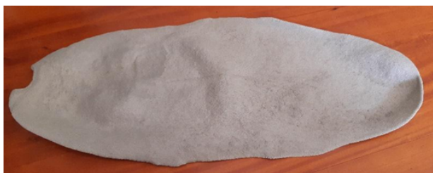
Figure 2: The compound before vulcanization
