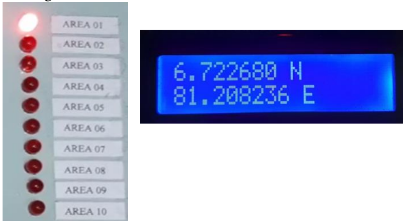
Figure 9: Turns on relevant area indicator and LCD display shows GPS coordinate
