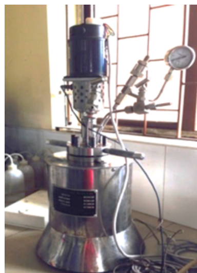
Figure 1. TOPT-50 mL high pressure reactor used in advanced experiments.
