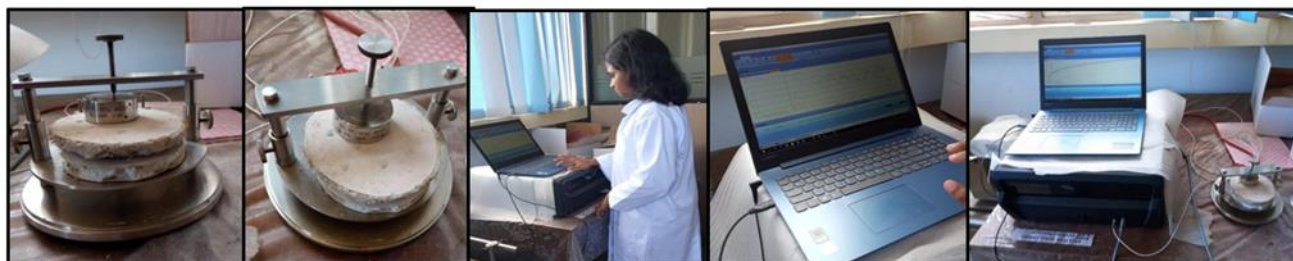
Figure 2: Thermal Conductivity Test Process (Source: Author, 2023)
