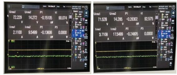
Figure 11 - Efficiency Measurement of the LLC Resonant Converter at Various Output Power Levels, Performed with a Power Analyser
