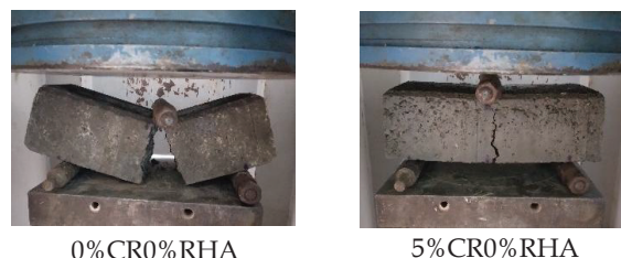
Figure 9 - Failure modes of flexural strength test
