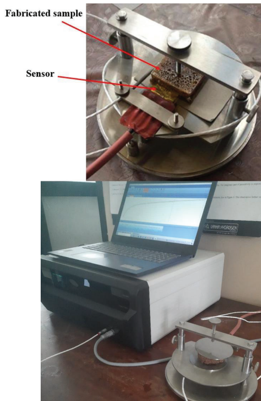
Figure 4 - Thermal conductivity measurement obtained by hot wire analyser in the Open University, Sri Lanka
