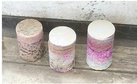
Figure 2 - Extracted Concrete Core Samples
