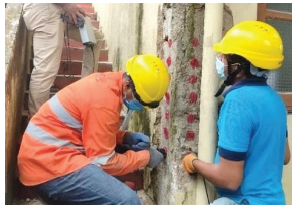
Figure 6 - UPV Test on a Reinforced Concrete Column
