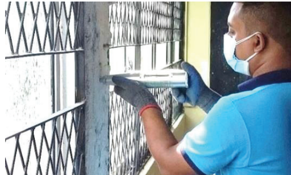
Figure 3 - Rebound Hammer Test on a Reinforced Concrete Column
