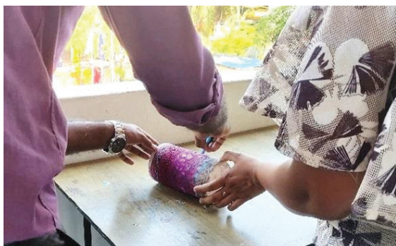
Figure 5 - Marking the Carbonated Area on an Extracted Core Sample
