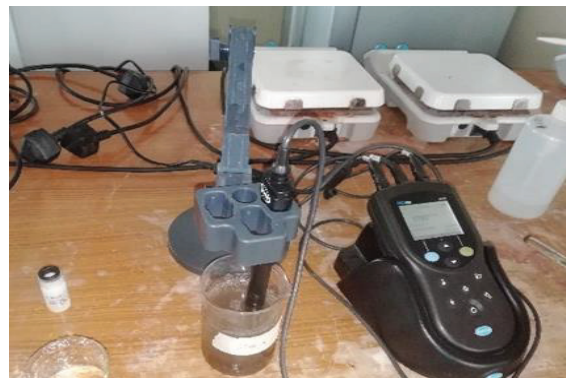
Figure 4 – Measurement of Electrical Conductivity of MSW Samples
