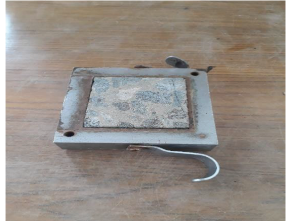
Figure 5 - Concrete Sample was Placed at the Bottom of the Shear Box
