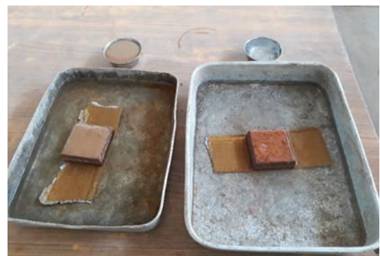
Figure 6 - Soil Samples with Drilling Liquid kept for Saturation
