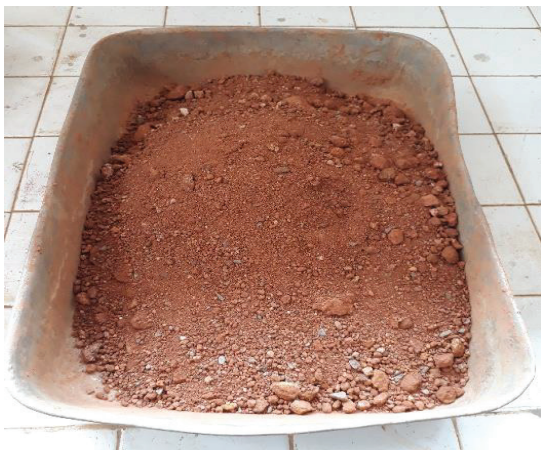
Figure 1- Laterite Soil used for the Experiment
