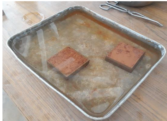
Figure 3 - Soil Samples kept Submerged in Water
