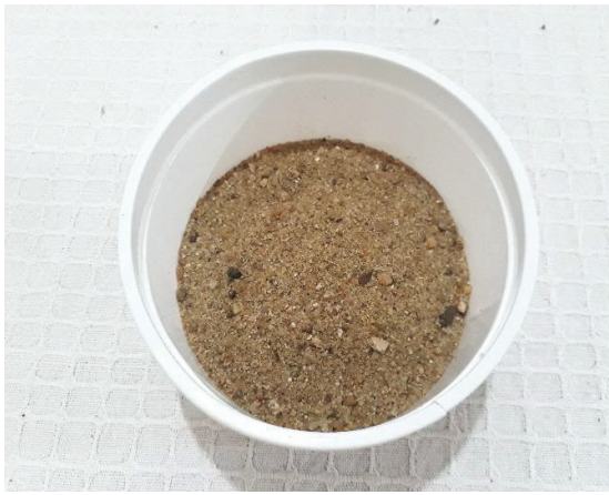
Figure 4 - Commercially Available River Sand
