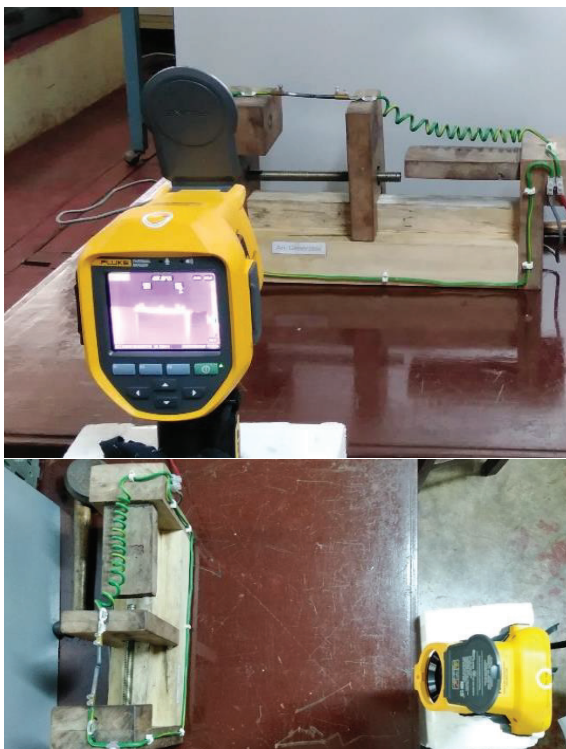
Figure 11 - Physical Arrangement for Thermal Imaging
