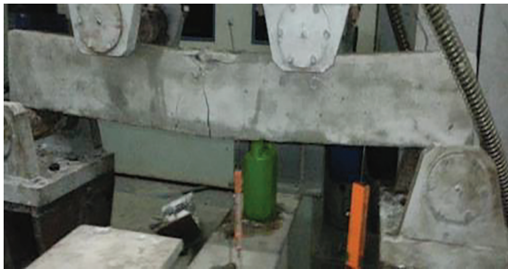
Figure 9 - Experimental Setup for a Flexural Capacity Test
