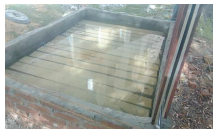
Figure 4 - Specimen Subjected to Accelerated Corrosion in NaCl Pond
