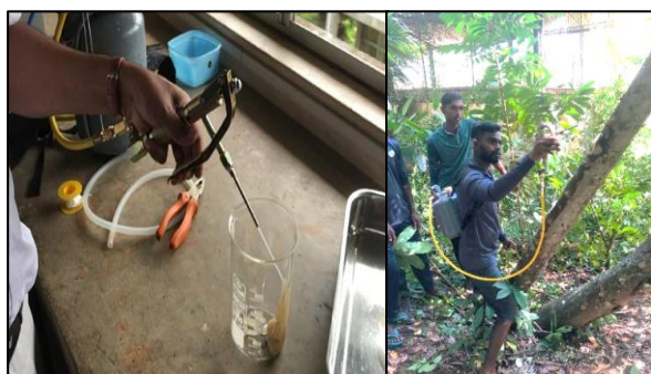
Figure 2: Discharge Testing with Different Pressure Levels
