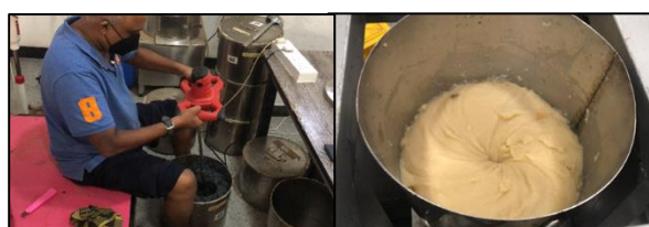
Figure 8: Mixing process by hand held motor driven by agarwood-inducing inoculum mixing machine
