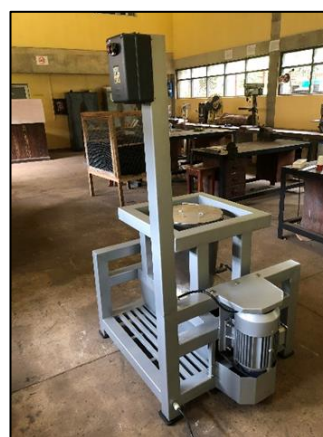
Figure 2: Agarwood-induce inoculum mixing machine
