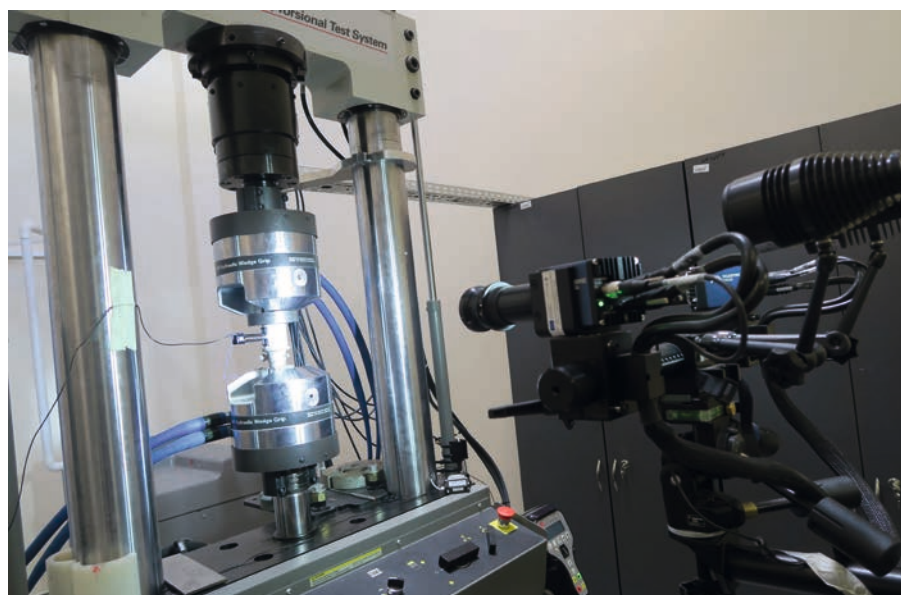
Fig. 6. Measurement of \epsilon_{xy} deformation of the sample using the ARAMIS 3D 4M vision system (photo by author)
