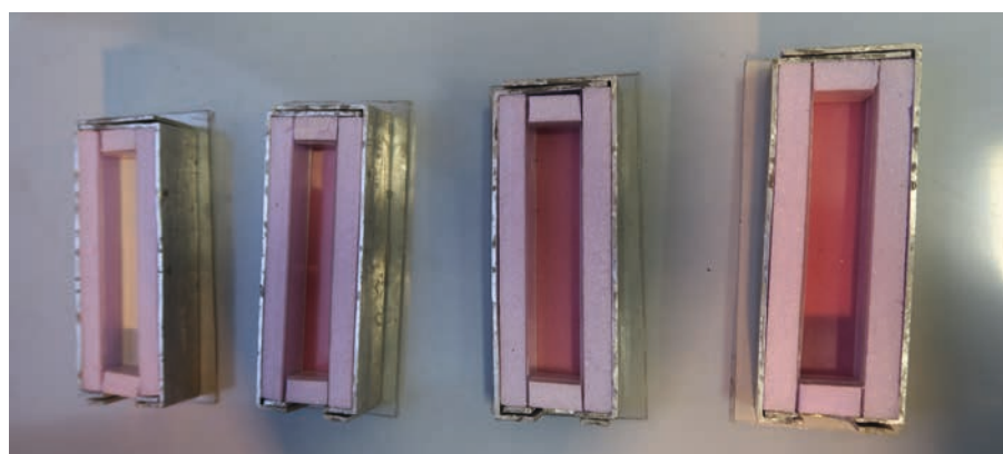
Fig. 7. Forms for preparing 10 x 10 x 80 mm polyurethane adhesive samples (photo by author)
