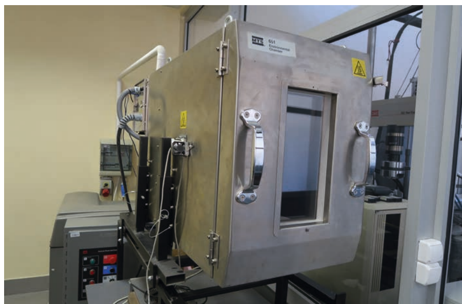
Fig. 8. MTS 651.05E-02 environmental chamber with assembly platform (photo by author)
