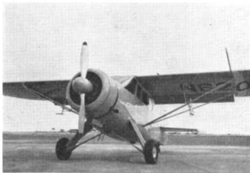
Fig. 1. Howard aircraft used to obtain observations windward of the Island of Hawaii. The liquid water content sensing unit is beneath the port wing. The vortex thermometer under the starboard wing was replaced by the psychrometer unit during "Project Shower".
