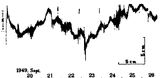
Fig. 4. An example of records obtained with a highly sensitive gravity variometer of double bifilar suspension type (sensitivity: 1 \times 10^{-8} \text{ g/mm/2 m} ).
