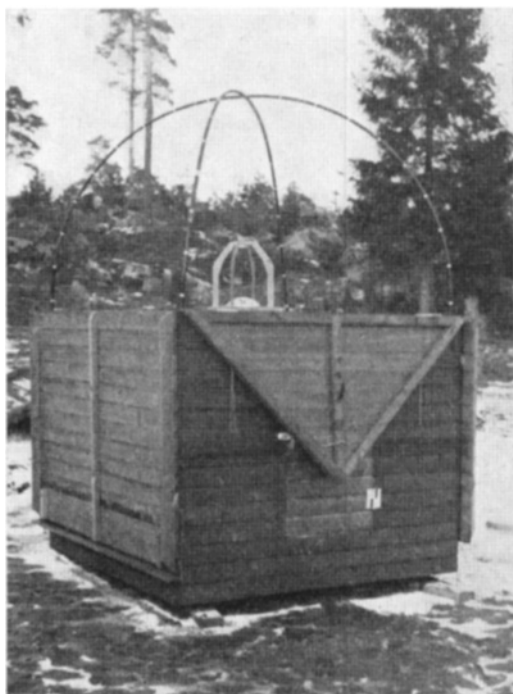
Fig. 4. The complete camera arrangement opened for observation. Figures 5 a, b show the arrangement of the mirrors and figure 6 shows the optical details.
