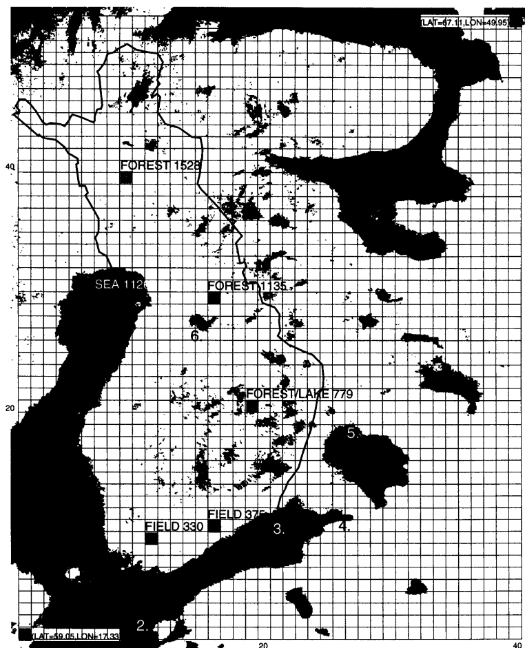
Fig. 2. The grid network based on 24 \times 24 pixel squares and the location of the selected test squares representing land surface types. The control points for testing the accuracy of the relative positioning of sequential images are numbered from 1 to 6.
