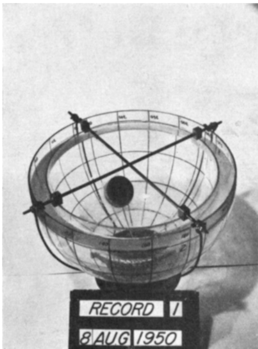
Fig. 1. Spherical apparatus adapted to the obstacle experiment.
