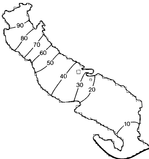
Fig. 6. Calculated structure of the first mode of the Adriatic Sea with a period of 21.9 h on the high resolution grid with no rotation. Solid lines are co-range lines relative to a maximum of 100.
