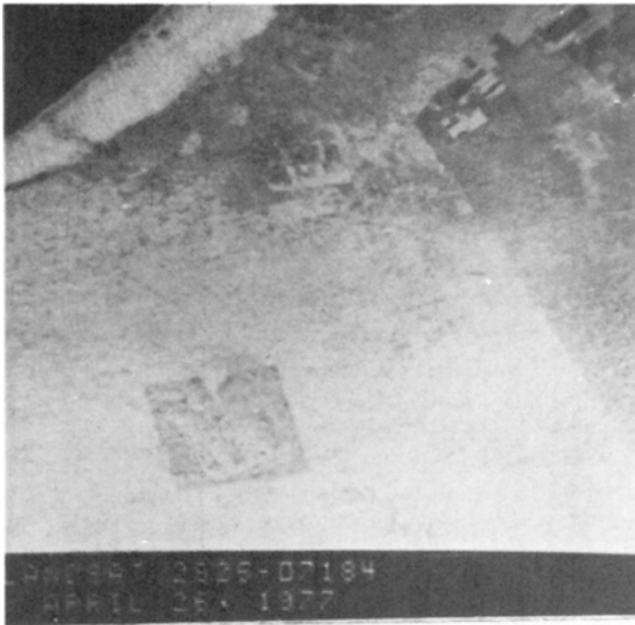
Fig. 1. The western Negev and the northern Sinai, part of Landsat image E-2 987-07100, in reflective infrared band MSS-6, 0.7\text{--}0.8\ \mu\text{m} . The Negev (on the right) and the enclosure (a square area 5.5 \times 5.5\ \text{km} , in the middle) show up as dark in sharp contrast to the bright Sinai (surrounding the enclosure). The Mediterranean Sea is on the left. Approximate scale 1:500 000; October 5, 1977, sun elevation 41.5^\circ .
