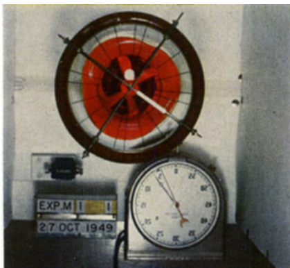
Fig. 7. Three-crest pattern observed when fan is rotating faster than bowl at a moderate rate. The crests progress relatively cyclonically at a rate equal to about .16 of the bowl rate of absolute rotation. (Apparent rotation of bowl counterclockwise, bowl absolute rotation 56.4 rpm, fan rate +30.1 rpm relative cyclonic, \gamma = 0.096 with chlorobenzene as lower liquid.)
