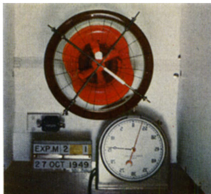
Fig. 8. Two-crest pattern observed when the fan is rotating faster relatively than in fig. 7. The crests progress relatively cyclonically at a rate equal to about .20 of the bowl rate of absolute rotation. (Apparent rotation of bowl counterclockwise, bowl absolute rotation 56.4 rpm, fan rate +41.4 rpm relative cyclonic, \gamma = 0.096 with chlorobenzene as lower liquid.)
