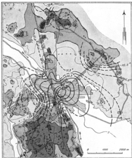
Fig. 7. Isotherm map for February 25, 1948, around 0600 hours. Cloudiness: 0. Wind: SW 1.5 m/sec. Absolute humidity: 1.9 mm. Relative humidity: 91 %. Ground completely covered with snow.
