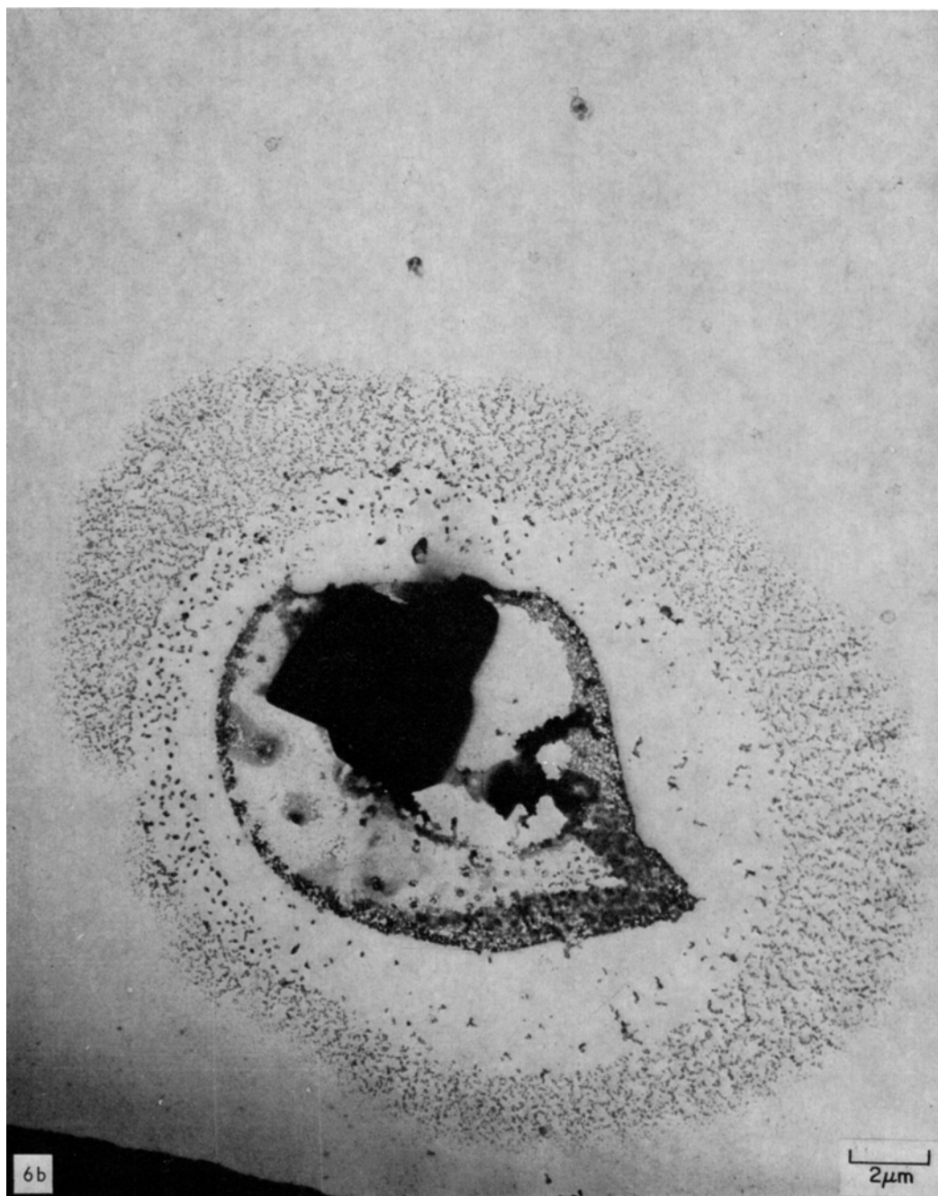
Fig. 6b. A typical sulphate reaction. The dark mass in the central region is unreacted sodium chloride, while the sulphate in the particle has reacted with the barium chloride deposit to form a halo of barium sulphate.
