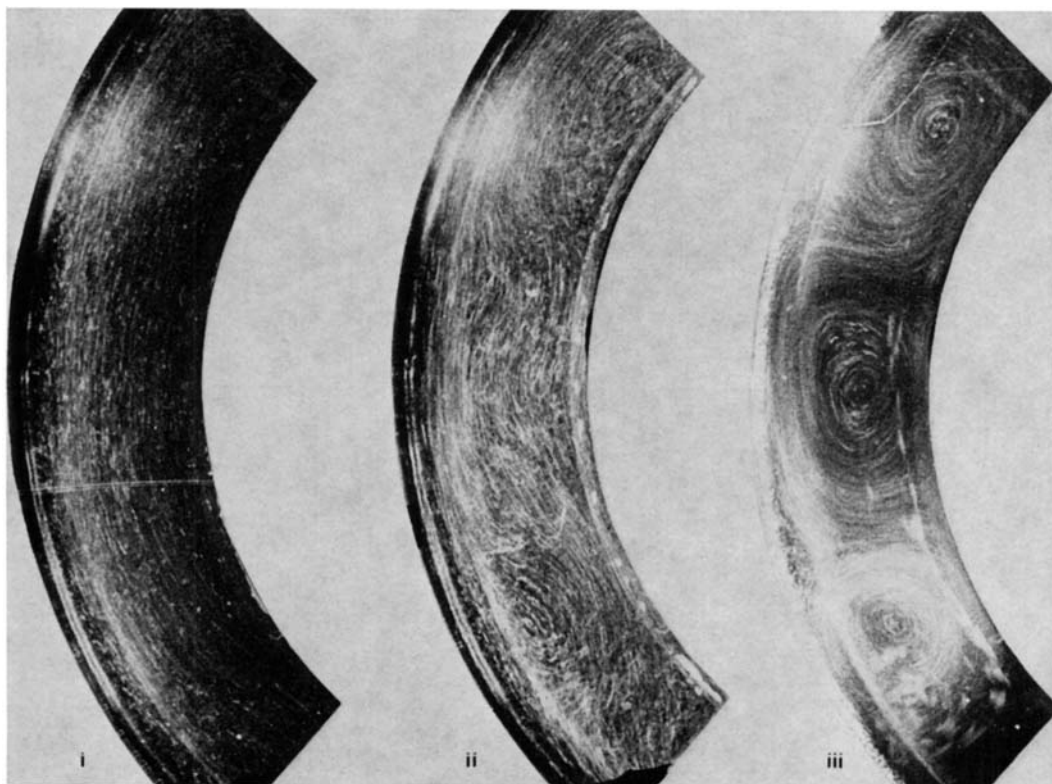
Fig. 10. Plan photographs showing the transition to the wave regime for the rigid lid case. All photographs are taken at the same depth in the fluid with an exposure time of 30 sec. The value of \Delta T = 20^\circ\text{C} and \Omega = (i) 0.49 rads/sec, (ii) 0.58 rads/sec, (iii) 0.79 rads/sec, and (iv) 1.91 rads/sec.
