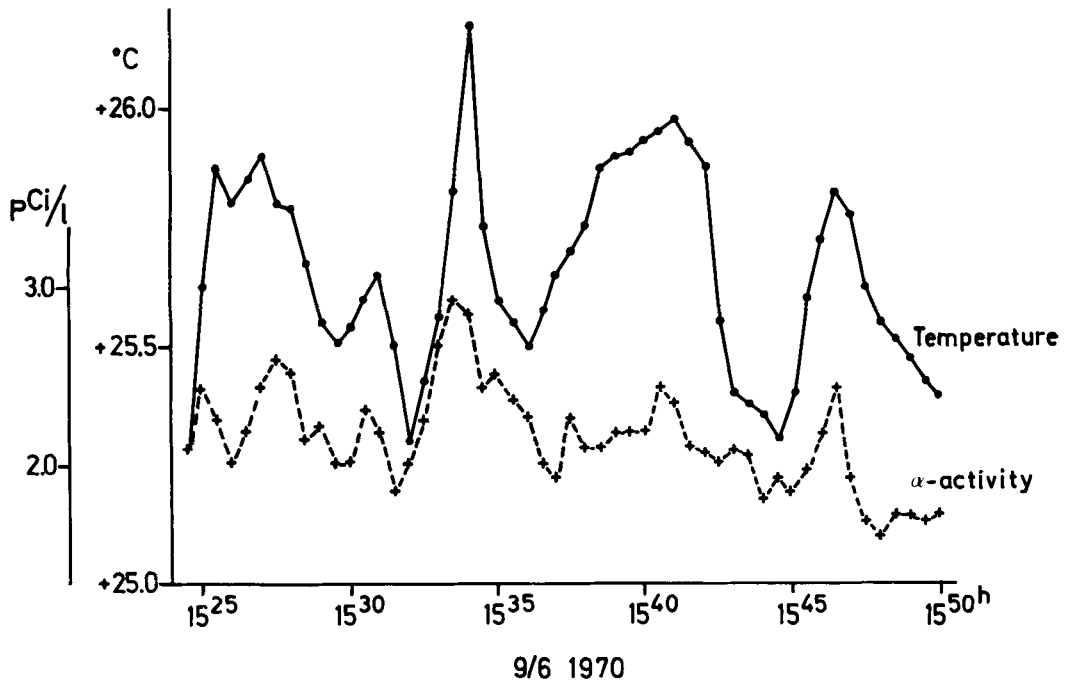
Fig. 5. Simultaneous fluctuations of natural \alpha -activity and temperature on a clear day in summer.
