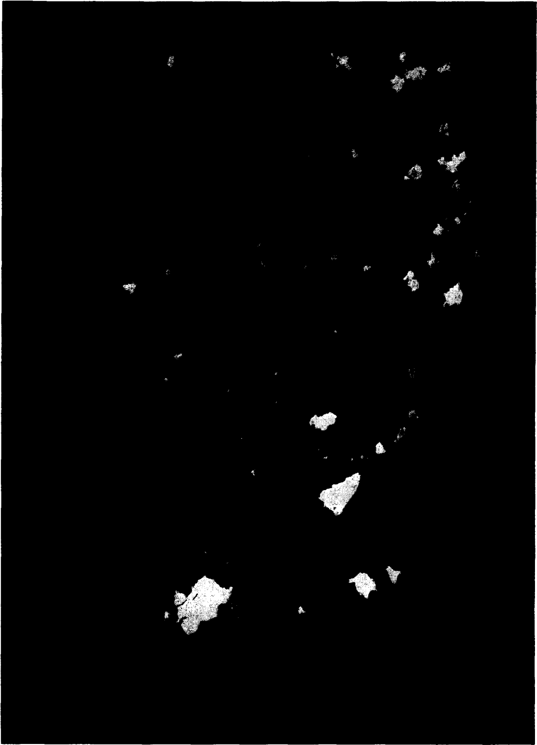
Fig. 8. The remains of an impact of a large particle collected by a "whirling arm" impactor.
