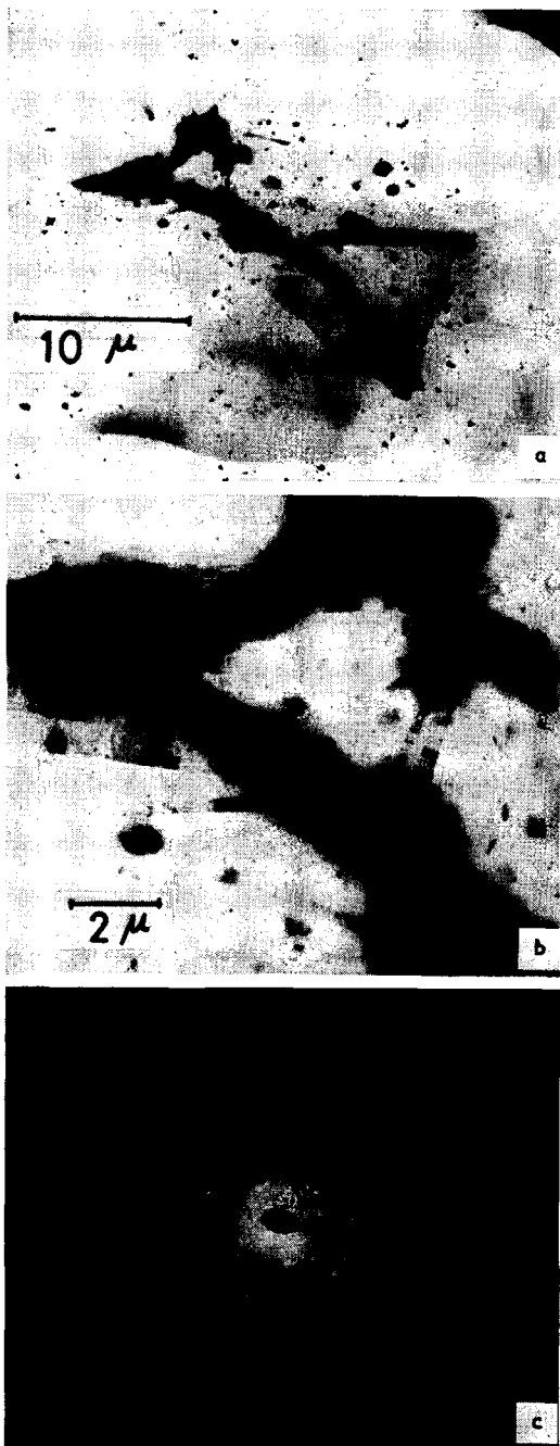
Fig. 21. (a) Particle of \text{CaSO}_4 and tiny carbon particles on 22 February at College. (b) A part of the particle of \text{CaSO}_4 in higher magnification which gives spot pattern (c) of \text{CaSO}_4 .
