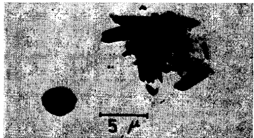
Fig. 10. Ice nucleus (clay mineral) on 14 February at Nagoya and condensation nuclei around it.
