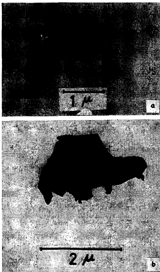
Fig. 27. (a) and (b) Ice nuclei (clay mineral) on 9 February at Mauna Loa. No other tiny particles are seen.
