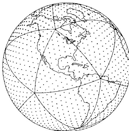
Fig. 5. Spherical geodesic grid with pole near the center of a major spherical triangle.
