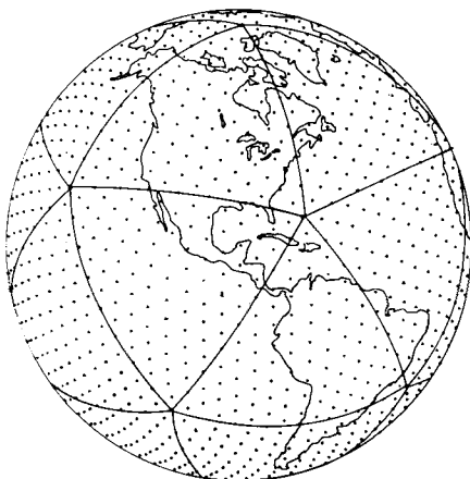
Fig. 4. Spherical geodesic grid with pole at a major triangle vertex.
