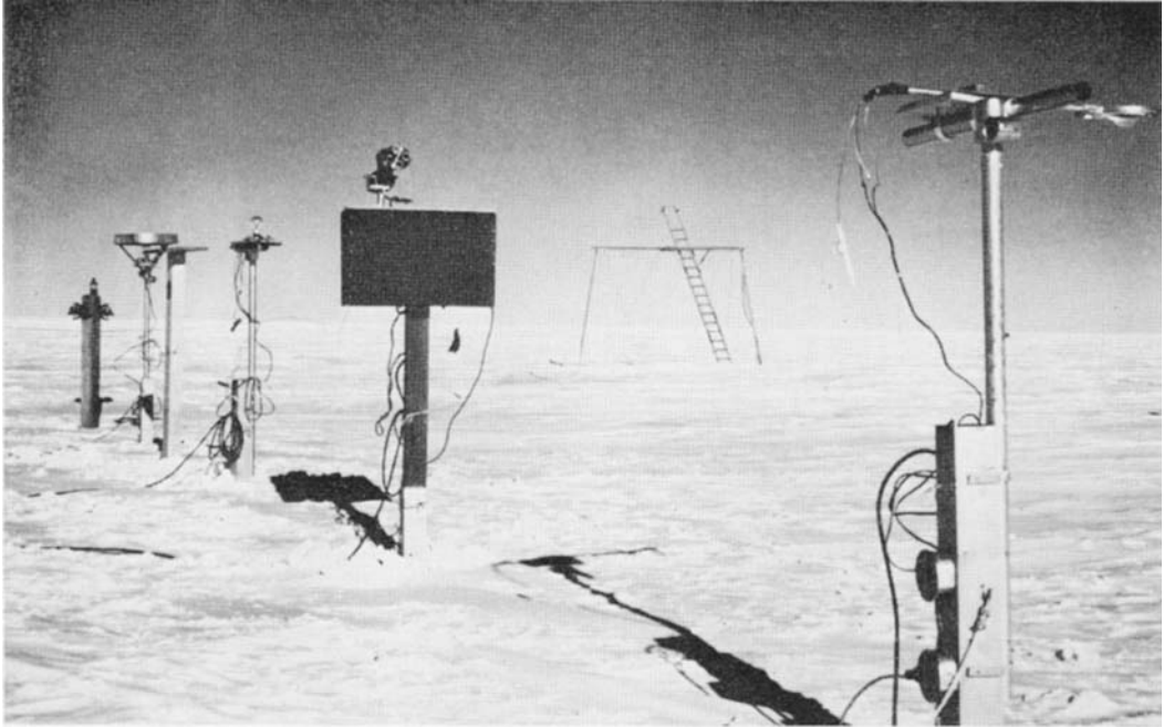
Fig. 1. The South Pole radiation instrumentation. From left to right: Campbell Stokes sunshine recorders, Eppler pyranometer with shade ring, empty platform, upfacing Eppler pyranometer, Eppler pyrhelimeter with filter collar, downfacing Eppler pyranometer, and CSIRO (Funk) radiometer.
