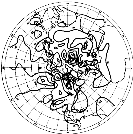
FIG. 15. The initial ( t=0 ) distribution at 00 GCT, 7 December 1957 of the stability \sigma , obtained with the two-layer variable stability model. The units are deg.
