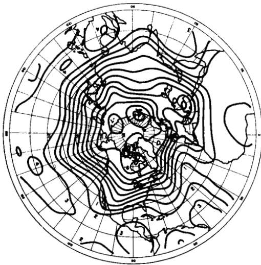
FIG. 4. The initial ( t=0 ) distribution of the streamfunction \psi , obtained from (44) with \psi=0 at the equator. The labeled units are 10^7 \text{ m}^2 \text{ sec}^{-1} .
