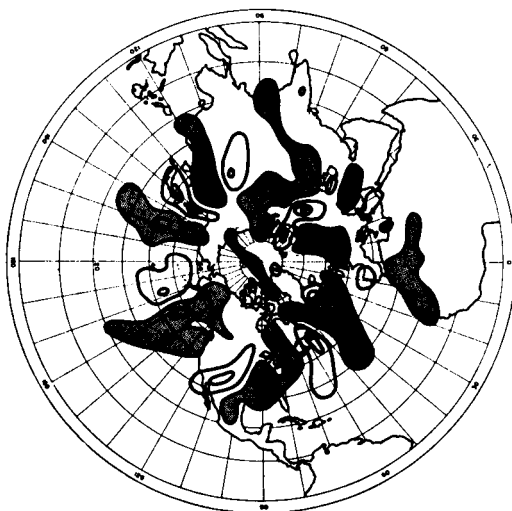
FIG. 8. The initial ( t=0 ) distribution at 00 GCT, 7 December 1957 of the vertical motion \omega , obtained with the quasi-geostrophic two-level model (47) with \omega = 0 at 5 N. The units are \text{mb hr}^{-1} . The isolines -5, -1, 3, 7, \dots are drawn, with the area of \omega more negative than -1 shaded.
