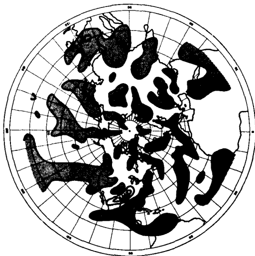
FIG. 19. The forecast distribution of the vertical motion \omega from the two-layer variable stability model, for 00 GCT, 8 December 1957 ( t=24 hr). The units are \text{mb hr}^{-1} . The isolines -25, -1, 23, \dots are drawn, with the area of \omega more negative than -1 shaded.
