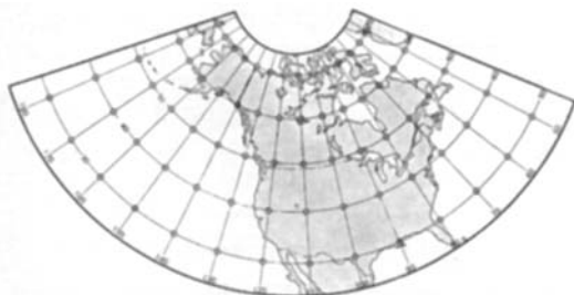
Fig. 1. Network of 70 grid points used to delineate the 700-mb height field. Heights were taken at standard intersections of latitude and longitude, 10 degrees apart, marked by open circles.
