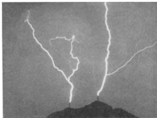
Fig. 6. Lightning flashes, starting from both towers, with upwards directed ramification. Tower distance 400 m, in direction of the figure 260 m. Visible channel-length 850 m.
