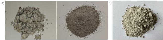
Fig. 1. Waste used in the study: a) bottom ash obtained from the incinerator, ground once in the mill (MSWI-BA); b) CBPD
