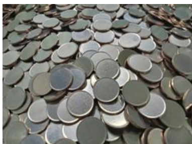
Fig. 6. Cupronickel-clad copper planchets prepared for minting trials
