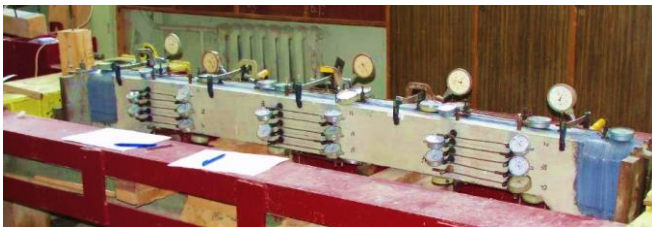
Fig. 4. Test stand with strengthened sample
