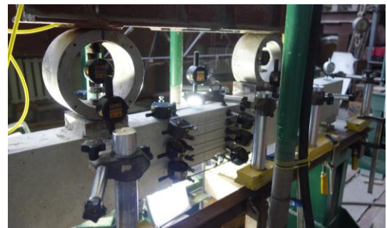
Fig. 4. Microtech measuring gauges were applied in the course of the experimental research
