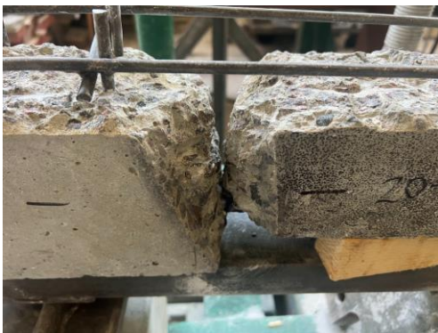
Fig. 6. Surface preparation and gap for restoration work
