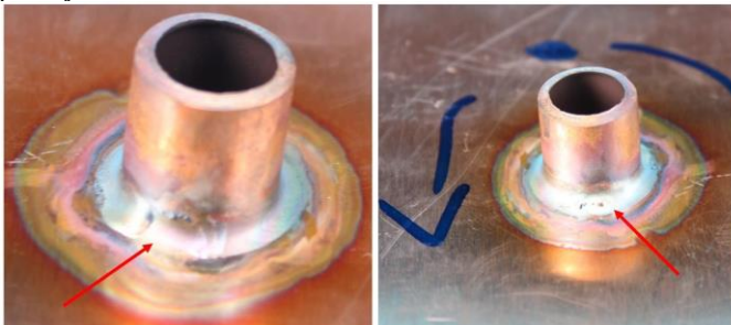
Fig. 14. Brazing seam overlap at start point (left) and interruption point (right)
