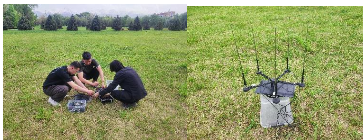
Figure 5. Experimental equipment setup and antenna array installed for direction-finding
