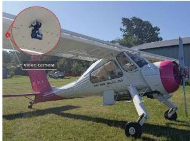
Figure 7. Photo of PZL-104 Wilga-35A aircraft with camera installed
