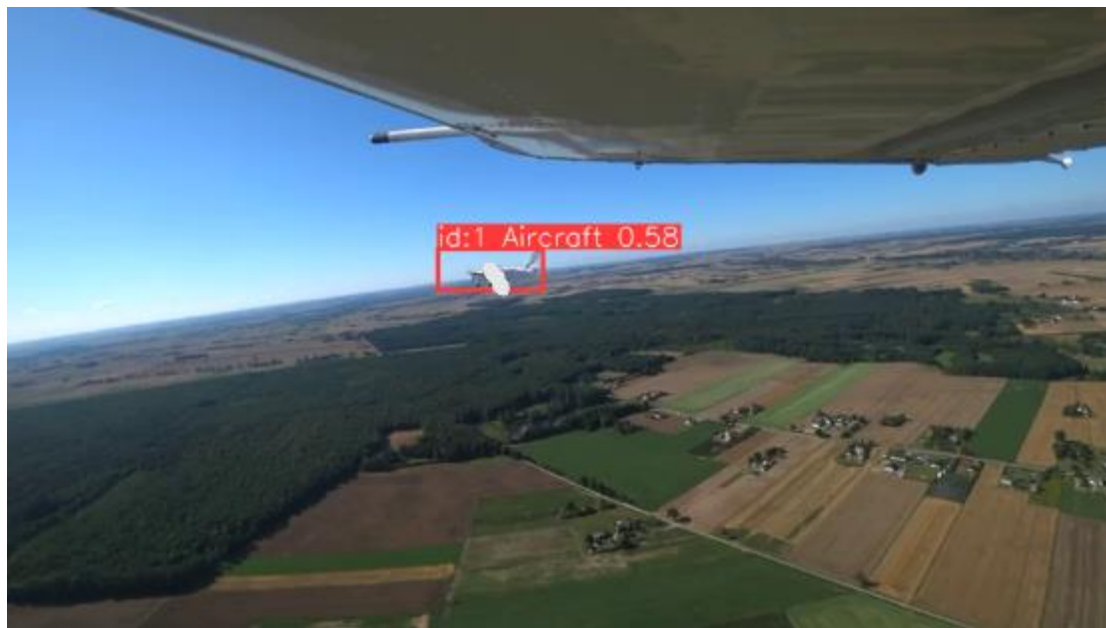
Figure 16. Example of the model inference and the use of the BoT-SORT algorithm
