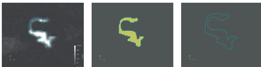
FIGURE 7. Left: the initial data and the isoline resulting from semi-implicit scheme. Middle: thresholding in Paraview and isoline of the semi-implicit method. Right: isolines of both semi-implicit and explicit (red) schemes, for this example almost identical.
