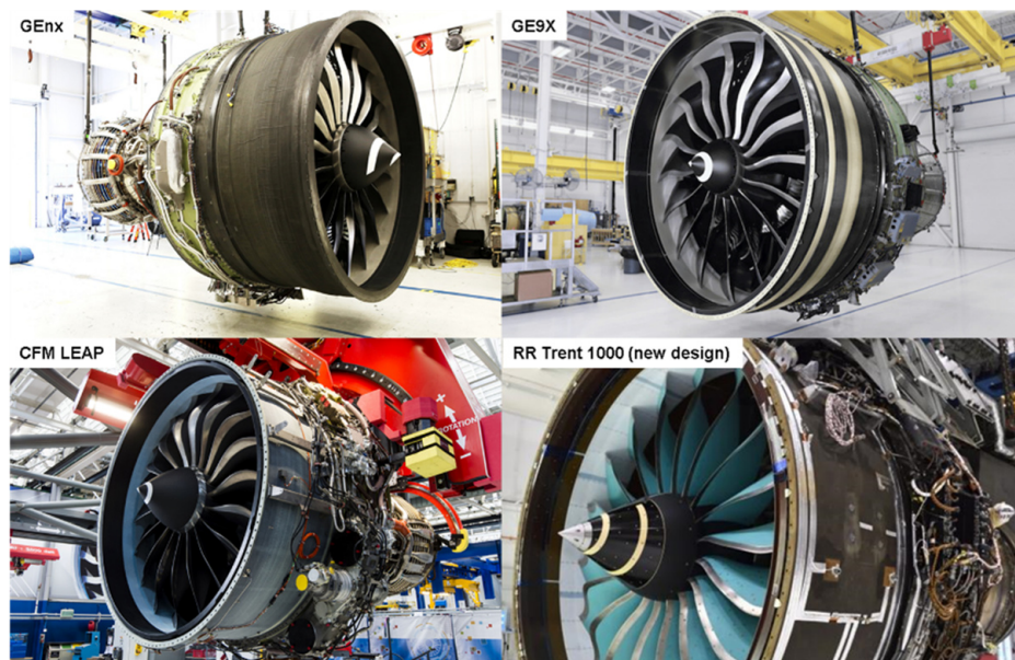
Fig. 1. Composite Fan Cases for high-bypass turbofan jet engines (GE nx [9], GE9X [10], CFM LEAP [11], RR Trent 1000 [12]).
