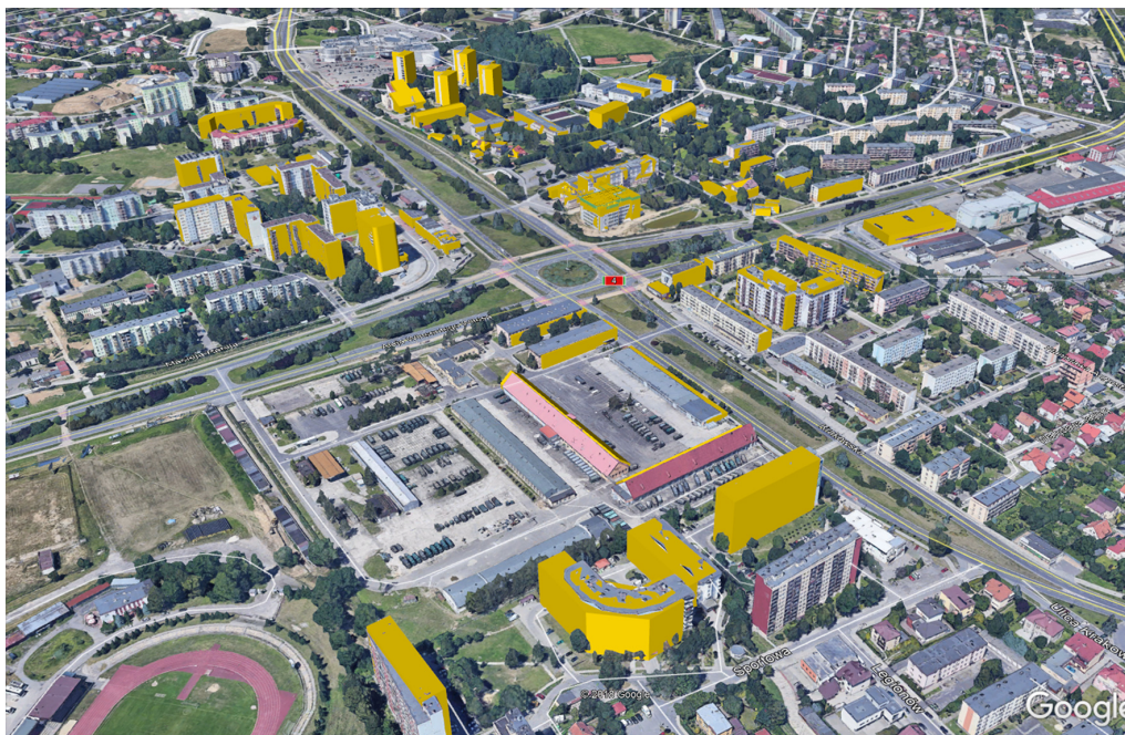
Fig. 33. Hospital in Rzeszów – overlapping LIDAR (textured) and 3D (yellow) model of whole city blocks.
