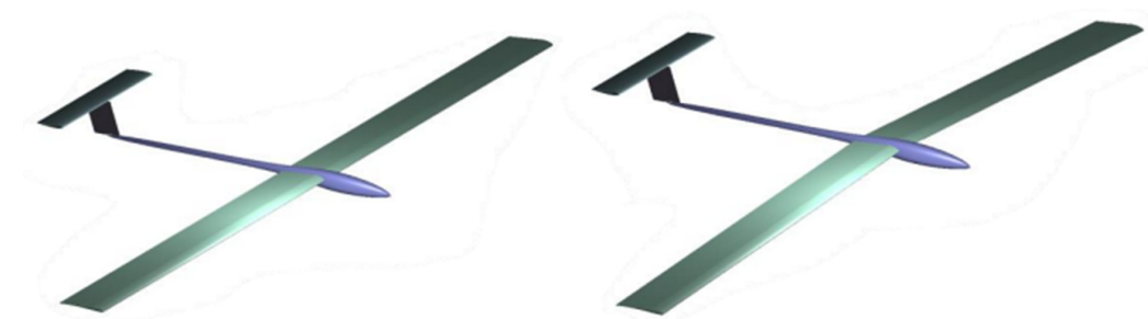
Fig. 4. Sketches of the jig shape of the solar UAV under analysis. Dihedral angle: 0 deg, -3 deg.
