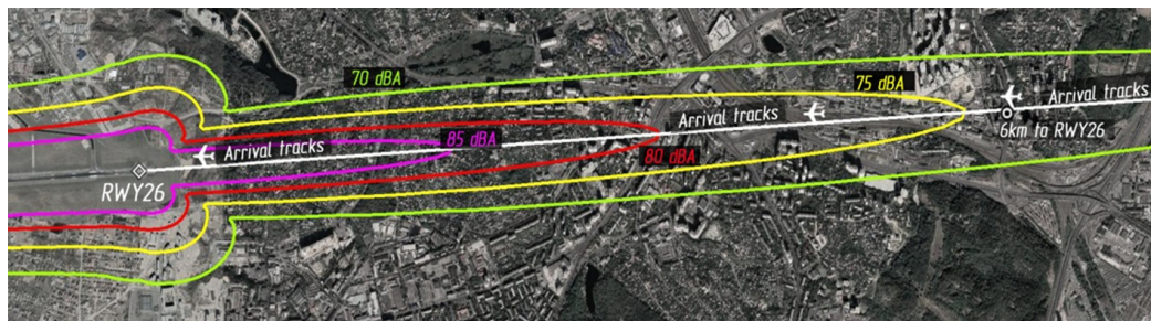
Fig. 7. Track dispersion (white lines) during descent and arrival procedures, typical for city airports; 70–85 dBA are L_{Amax} noise levels.
