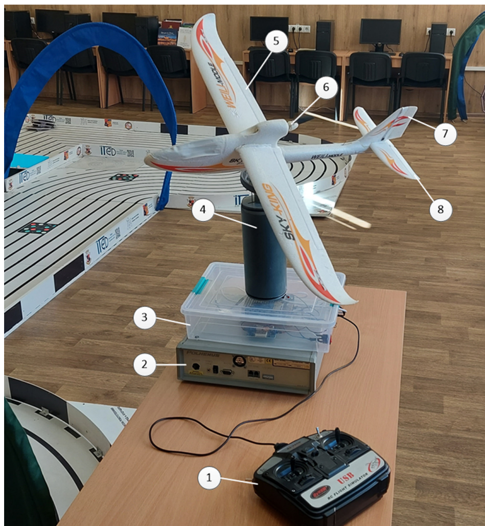
Fig. 2. Physical model of the flying object in one of its positions in space. The following designations are accepted in the Fig. 2: 1 – remote control; 2 – microprocessor module; 3 – power block; 4 – booms; 5 – airplane flaps; 6 – airplane propeller; 7 – rudder; and 8 – elevators.
